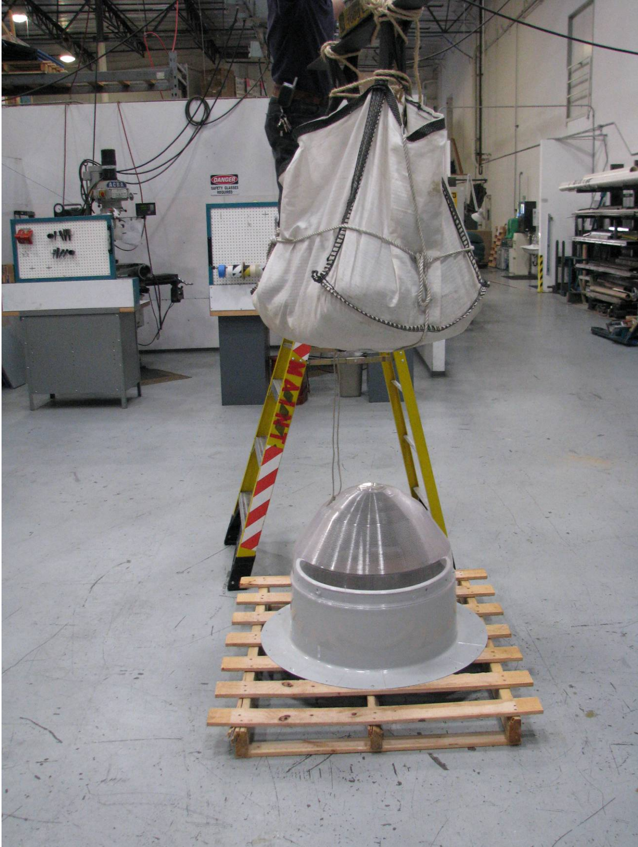
Photo No. 4 Sand bag at drop height
