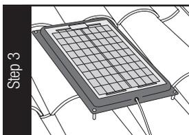
**Step 3:** Secure the solar panel to the tile roof using the four (4) 2" screws provided. Insert two (2) 1" standoffs on the dow Re-connect the panel to the Y-Connector. Connect the new Add-on Panel to the Y-Connector. NOTE: RED wires connect to RED terminals only, and BLACK wires connect only to BLACK terminals. For final connection, see diagram for Step 3E.
