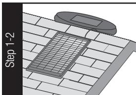
**Step 2:** Using the four (4), 2" (51mm) screws provided, secure the solar panel to roof through the four pre-drilled holes in mounting plate. Coat screws with sealant (not provided). Route 15' (4.5m) power cable to either Solar Star Roof Mount Vent or Solar Star IM 1200.
