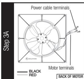
**Step 3D-3E:** Disconnect one lead wire from motor terminal at a time. Add a Y-Connector to the BLACK and RED motor leads. Re-connect the panel to the Y-Connector. Connect the new Add-On Panel to the Y-Connector. NOTE: RED wires connect to RED terminals only, and BLACK wires connect only to BLACK terminals.
