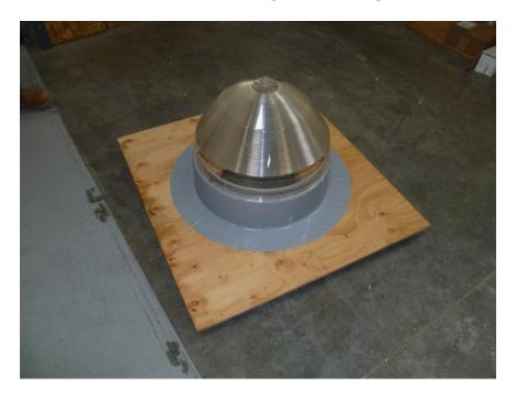
Photo No. 2 750 DS TDD after static loading
