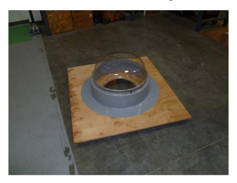
Photo No. 4 330 DS TDD after static loading
