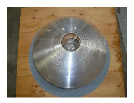
Photo No. 3 750 DS TDD after static loading
