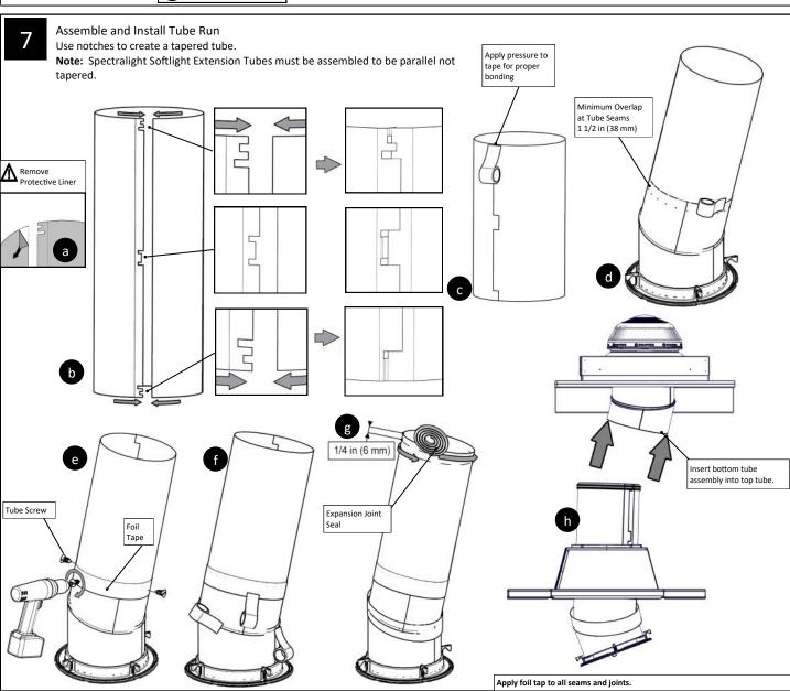
**Note:** Install Spectralight Softlight Tubing at bottom of tube run for best results. Use no more than one (1) Softlight Extension Tube for each assembly.
