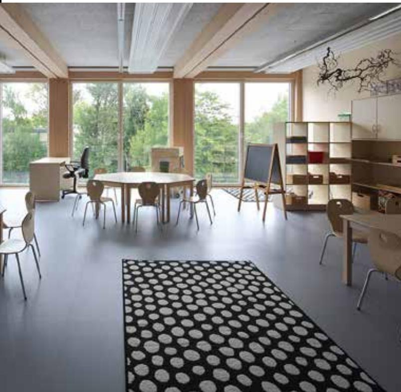
Each classroom is 870 square feet and is made up of three prefabricated wood modules.
