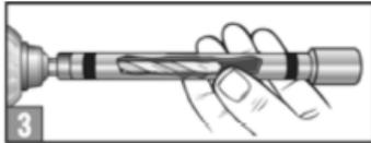
**Step 3:** Place Condribe® tool with drive socket over drill bit.
