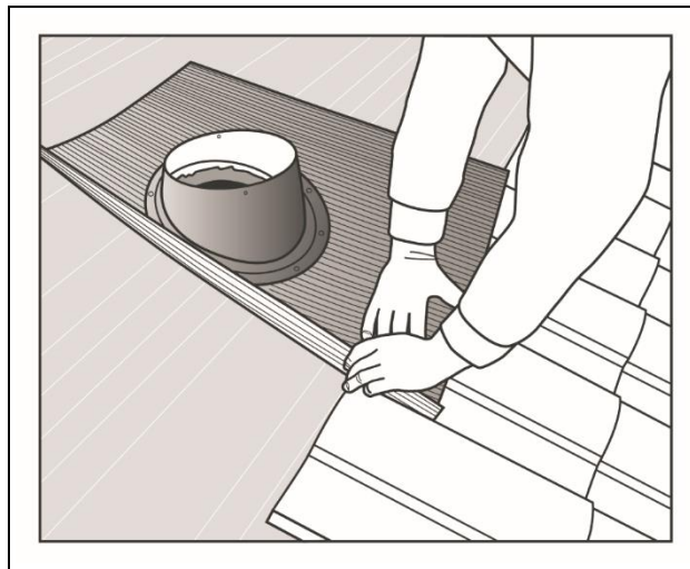
Figure 8 Securing the interlocking tile flashing
